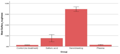
Fig.1. Means and standard deviations of the tested groups' surface roughness ( $\mu$ m).
