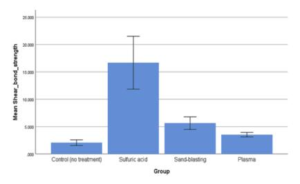
Fig.2. Means and standard deviations of the tested groups' shear bond strength (MPa).
